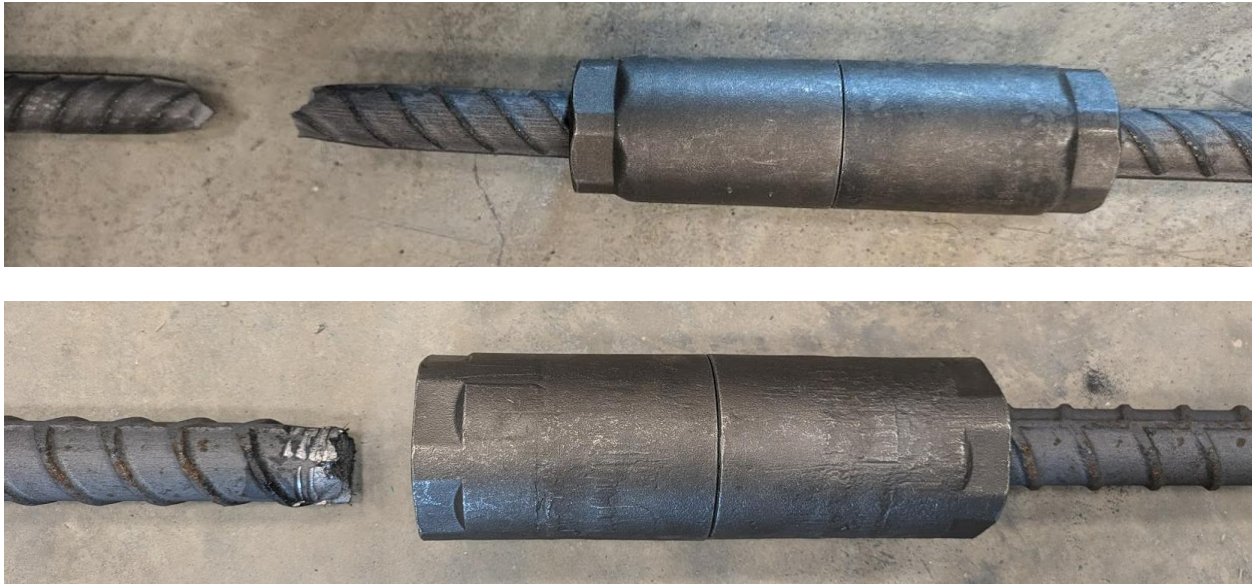
Figure 3. Representative fractured spliced bar test specimens. Top: Bar fracture away from the coupler. Bottom: Bar fracture at indentation in bar created by the wedges internal to the coupler.
